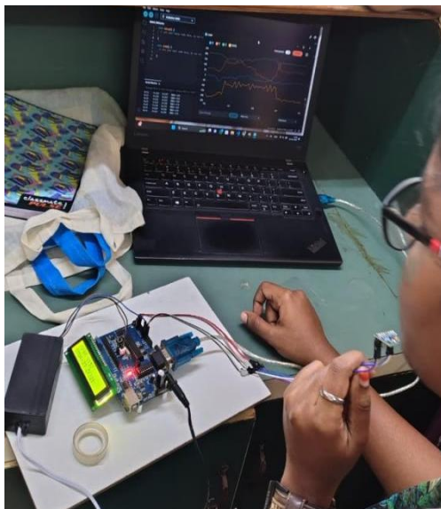
Figure 3: Real-time visualization of EMG and accelerometer signals using Arduino Serial Plotter.
